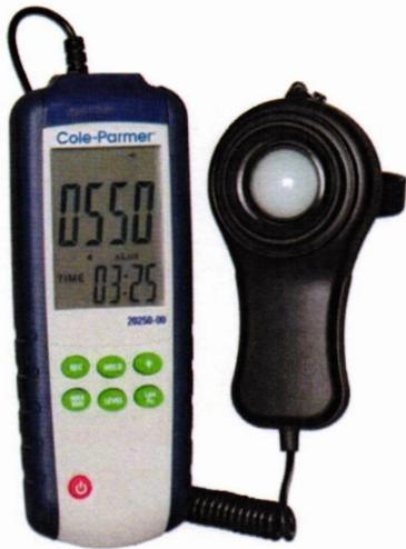
The Digi-Sense 20250-00 is a professional grade tool providing measurements in Lux or foot candles with a resolution of 0.01 Lux (much higher than the previously mentioned meter) and an accuracy of +/-3% at 10,000 Lux. It is NIST traceable. However, it is not reliable with all LED colors or technologies. This is a good, all around option, but the limitations with LEDs must be considered. The Digi-Sense 20250-00 costs about \$230.
