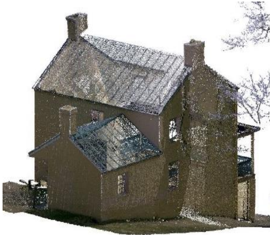
3D Point Cloud scanning of house (Mills Group 2018).
