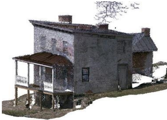
3D Point Cloud scanning of house (Mills Group 2018).
